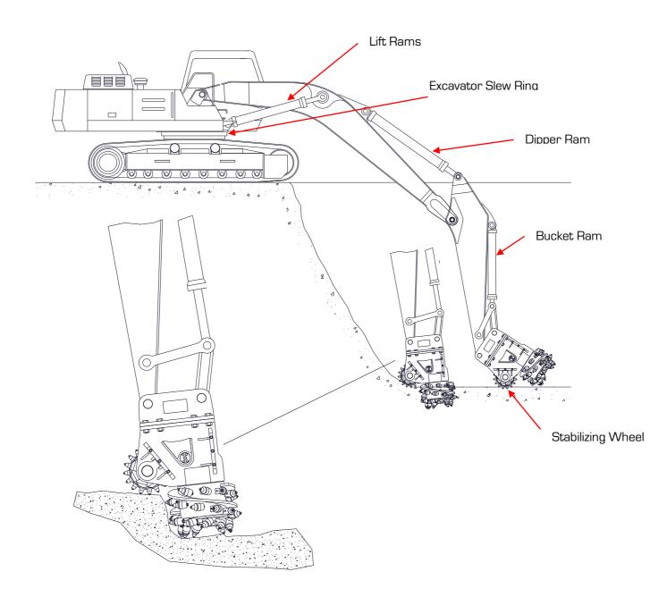
When the spoon cylinder is extended, the cutting unit is pressed into the ground, since the picks of the stabilizing wheel is supported in the ground.
